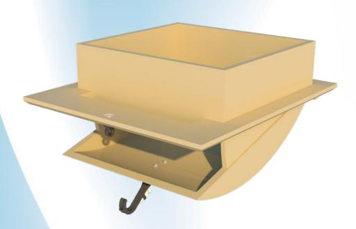
The 160-P-C air inlet valve is specially designed for installation in ceilings. This inlet is used to bring air from the attic into the different sections of the house. Working with ceiling inlets, in turn, helps to pre-heat the temperature of incoming air if necessary. The inlet is controlled by means of a central plastic arm.
