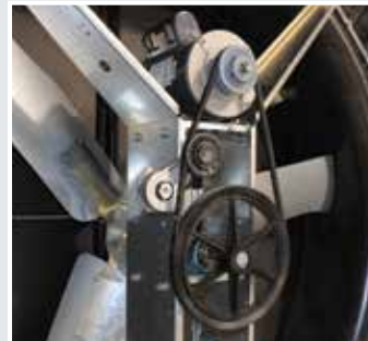
Standard, automatic belt tensioner and large, cast iron, greasable pillow block bearings for longer life.
