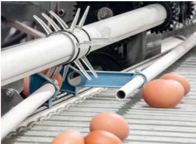
> Egg lift collection system - "Anaconda" chain
